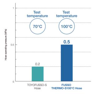
Test method: (Toyox standard test) All hose sizes shall be ø25. The hose operating pressure is the upper limit of the operating pressure shown in each hose standard table.
