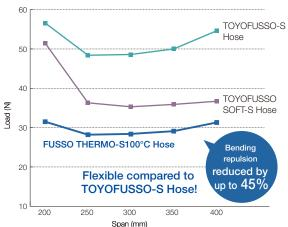
Test method: (Toyox standard test) All hose sizes shall be ø25. Compress and bend the sample hose as shown in the figure below, and examine the load for each set span and the load and span at the maximum load.
