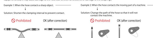
5. Perform piping and use hoses so as to avoid applying force to the base parts of the couplings.
